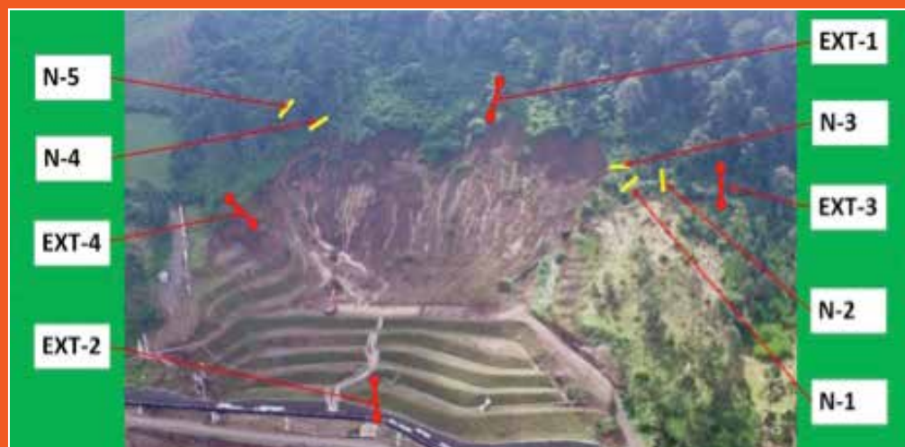
Example of Location and Distribution of Extensometer and Nuki-ita Monitoring Equipment at Landslide-1
